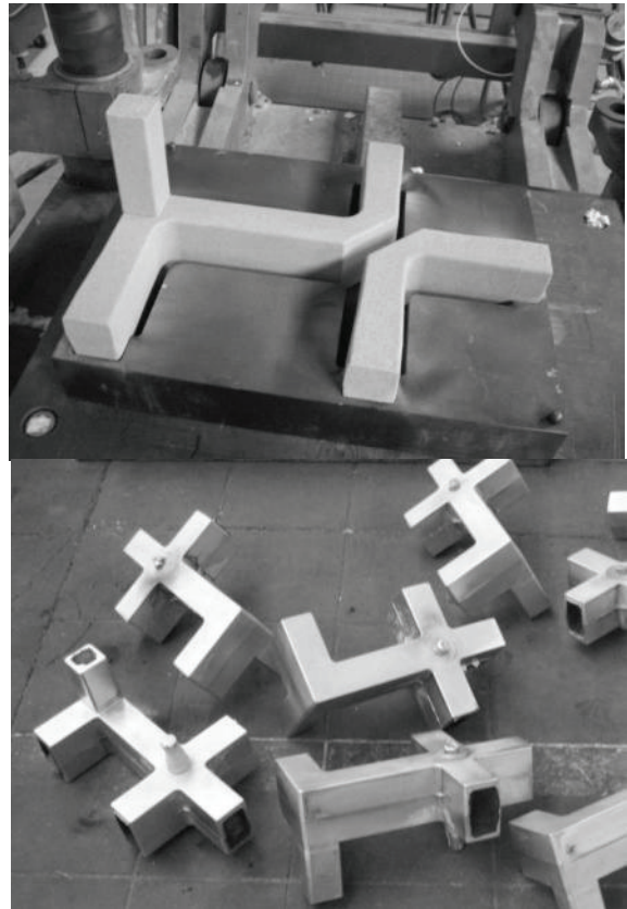
Fig. 9: Node A-column bottom, steel mold with sand core + castings
