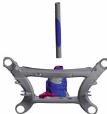
Fig. 8: Simulated rigid-body motion of the rear axle at 80 km/h
