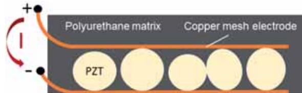
Fig. 4: Schematic structure of a sample (copper electrodes and PZT pearls in polyurethane matrix) and current flow through poling
