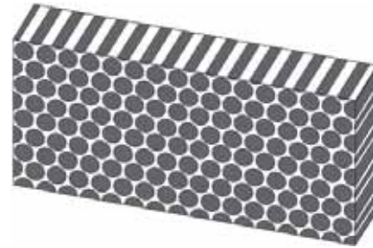
Fig. 8: Detailed quarter macro model of piezoelectric fiber composite; gray: piezo fibers; white: epoxy; electrodes are not visible in this graph
