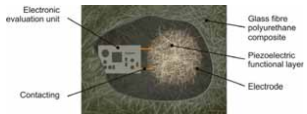
Fig. 1: Schematic of a fibre-reinforced polyurethane composite with integrated sensor elements
