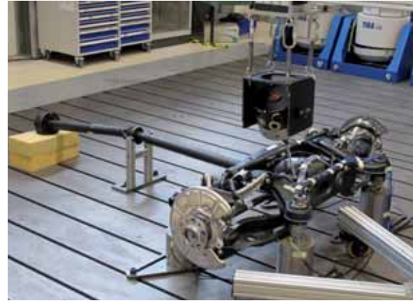
Fig. 9: Rear axle test bench with shaker excitation
