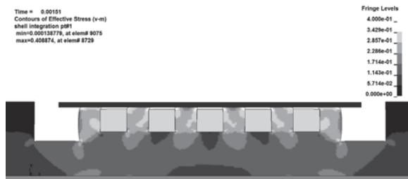
Fig. 10: V. Mises plastic equivalent stress in GPa of the aluminum sheet metal after joining
