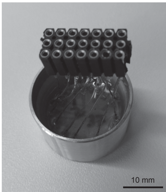
Fig. 7: Test device #37 with integrated piezo-composite for acoustic measurement
