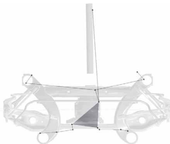
Fig. 4: Measured rigid-body motion of the rear axle at 80 km/h
