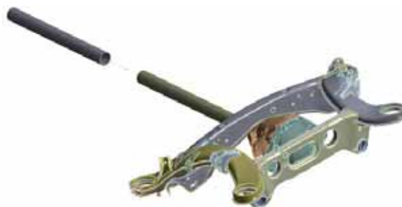
Fig. 7: FE simulation model of the rear axle
