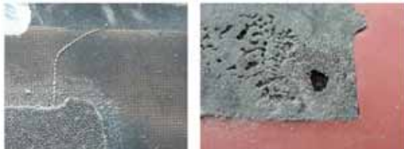
Fig. 6: Bypass wire (left) and electrical breakdown (right) resulting in unpoled samples
